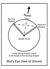
line using a pencil on a string and making an arc above and below the connecting line. Draw a line between the arcs. This line will point north and south. The direction away from the center of the circle between the shadows is the direction north.
