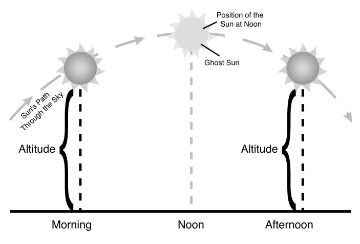
The morning altitude in degrees above the horizon must equal the afternoon altitude. The time exactly between equal altitudes is local noon.
