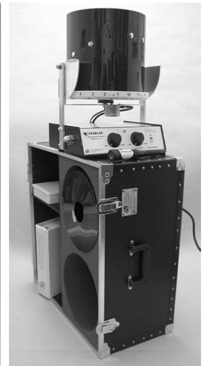
Shown above: the old-style Projector Travel Case as the projector stand in the dome. For systems shipped beginning in 2005, use the Blower or Cylinder Travel Case to achieve the correct projector height in the dome (see photo below).
