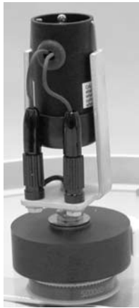
The banana plugs should be plugged in tightly.
